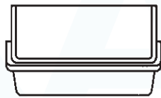
Bucket with front lip reinforcement
