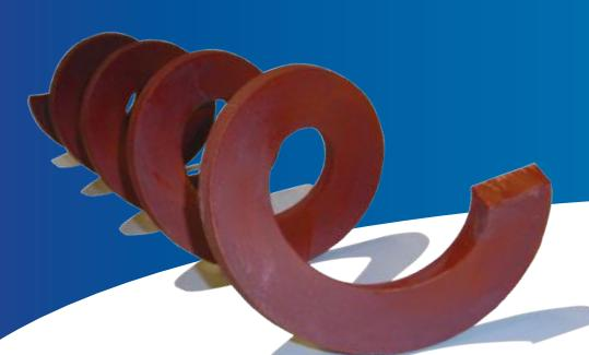
VAV supplies shaftless spirals in various lengths (material S355J2G3 or Stainless steel 304). Any desired size between Ø 80 and Ø 700 mm is available in single, double, triple and full sheet versions. Spirals can be used for horizontal, inclined or vertical transport. Suitable for wet, fibrous and sticky material. VAV also supplies auxiliary spirals in various sizes. The table below shows the standard sizes of shaftless spirals. Other sizes are available on request.
