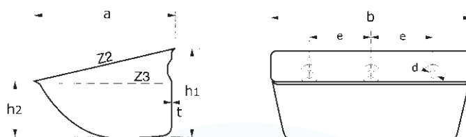
Super Starco elevator buckets in mild steel/stainless steel (parameters in mm)
